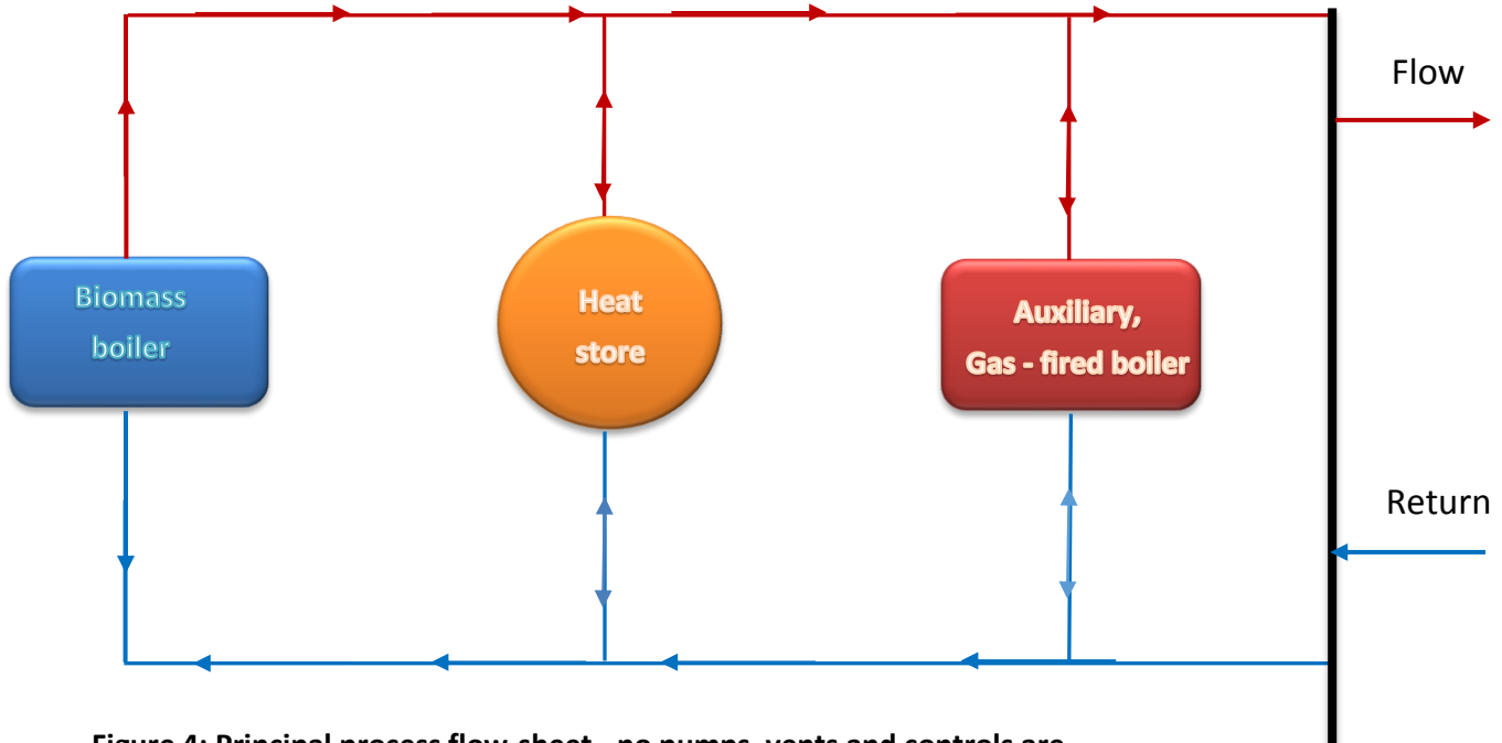
Figure 4: Principal process flow-sheet - no pumps, vents and controls are indicated
