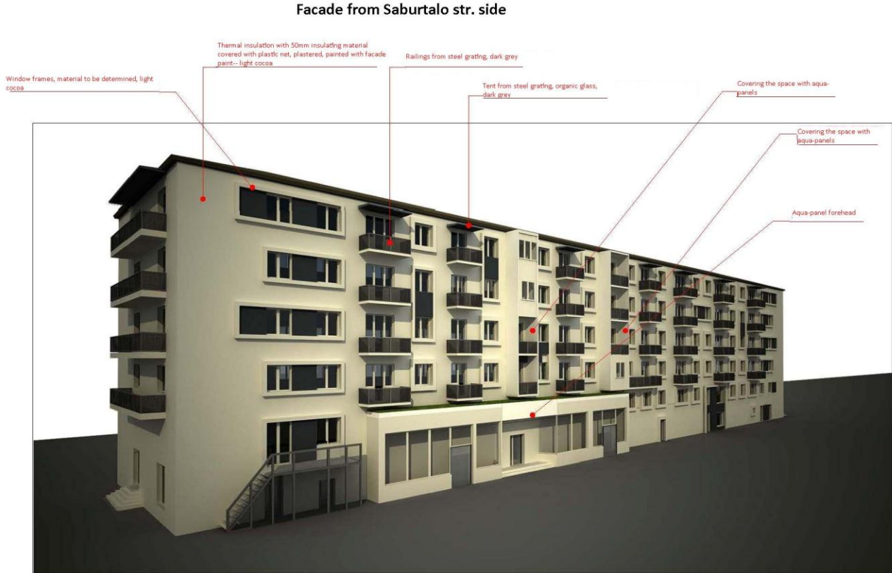
Fig 4. Façade from Saburtalo str. Side
