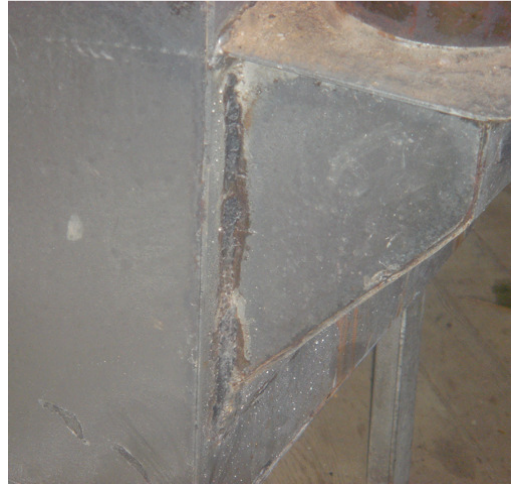
Figure 6. Typical welds and sharp edges on Georgia Industrial Group stoves.
