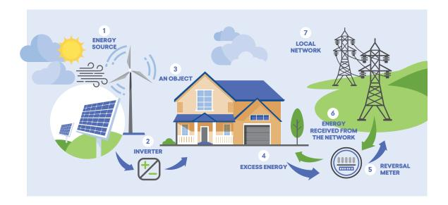
Electricity generation by the micro-generator and the consumption of the generated electricity can take place in different locations where it and its customer/group of customers are connected to the same distribution company. If the generation and consumption points are different from each other, both reverse meters and smart meters can be installed for each customer.
